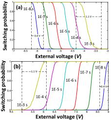
Figure 9. Voltage dependency of ON (a) and OFF (b) switching at different pulse widths  $t_{switch}$ .
