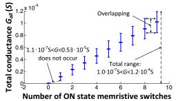
Figure 5. The conductance distribution of parallel connected memristive switches.
