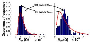
Figure 2. The static state distributions of a memristive switch.
